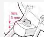
Ensure that the child seat is mounted at least 5 mm below the end of the tube.
