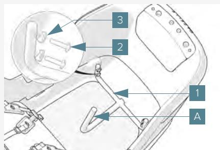
Position the adapter frame **1** with the vertical tube **A** as indicated in the diagram.
