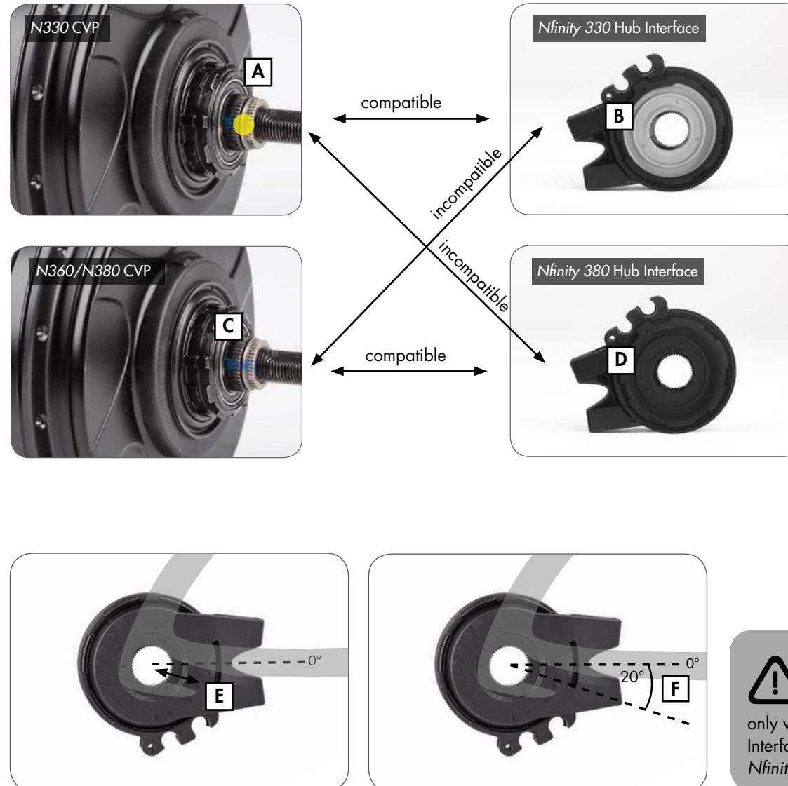
**⚠️** N330 and N360/N380 series CVPs have different shift driver configurations, and are compatible only with the appropriate *Ninfinity* Hub Interface. Do not attempt to fit incorrect *Ninfinity* Hub Interfaces, as damage will occur.
