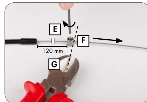
4. Cut the excess cable at a maximum of 2.0mm from the end of the UD cable stop (**G**).
